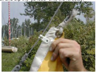
4. Attach the headstay wire to the head of the jib
