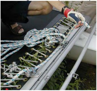
13. Pass the end of the main sheet through the pad eye and make a figure-8 stopper knot.
