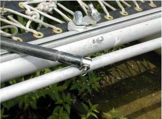
9. Attach the main halyard shackle to the head of the main sail. Feed the head of the main sail into the track opening on the mast. Do not raise the main sail until you have launched the boat.
