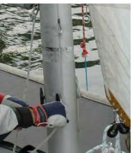
18. Insert and lower the gooseneck assembly of the boom into the mast track.
