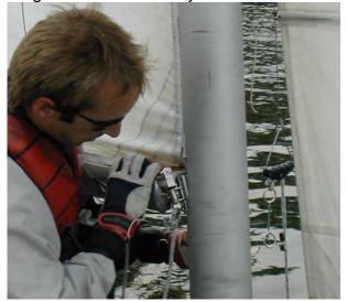
19. Tighten the downhaul to apply tension to the main sail. Tie off the downhaul on the mast horn cleat.
