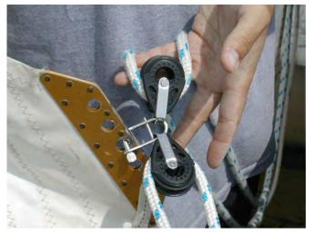
7. Pull on the jib halyard to raise the jibsail. The jib halyard line should wrap down around the fixed block at the bottom of the mast and then thread back up through the block on the halyard (to give more leverage). Raise the jib to tension the mast and the forestay should be slack. Tie off the halyard line on the horn cleat at the bottom of the mast. Coil extra line over the horn cleat.
