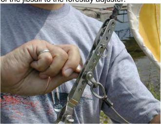
6. Attach the jib blocks' shackle to the clew of the jib sail. Ensure that the jib lines are not twisted.
