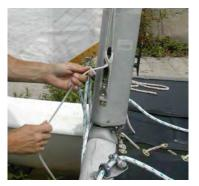
8. Remove the line that secures the tiller and attach the tiller extension to the hinge yoke on the tiller. Do this on land to ensure that you do not lose the clip. Tie the line to the trampoline so as not to lose it.
