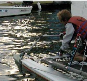
16. Fully raise the mainsail. Feed the luff of the sail into the track as you are pulling on the halyard. It may be helpful to pull the luff of the sail and/or the boom towards the
