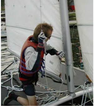
17. To "lock" the main sail at the top, it is necessary to pull the halyard towards the bow and center the metal "slug" on the halyard (the second slug) in between the two prongs of the "catch". Tie off the halyard line on the horn cleat at the bottom of the mast. Coil the extra halyard line and tuck it into the trampoline pocket (pass underneath the jib sheets).
